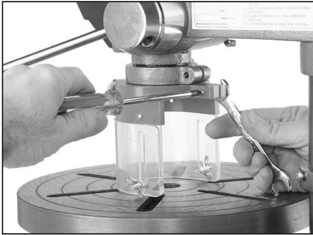
Figure 14. Installing chuck guard.
